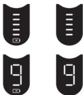
The **battery status** is shown with segments and additionally in digits (for some models also with a battery icon).
